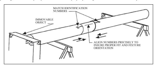
Cover the jam sleeve and the immediate inner section of the section that it will be fitted into with a light layer of liquid soap. Do not use grease, oil or other petroleum products as these lubricants can seep out over time and stain the flagpole. Keep the finish surfaces free of hand prints and excess lubricants.
